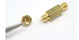
After separating the cap of the *TDR probe*, the pin can be inserted or not.
