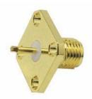
GigaLane SMA(Sub Miniature A) connectors are widely used in the frequency range DC to 18 GHz with low loss characteristics. SMA connectors are most used in military, microwave frequencies and telecommunication application.
