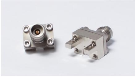
GigaLane High Performance End Launch Connectors are designed for 2.4mm (50 GHz), 2.92mm (40 GHz) and SMA (27 GHz) with Low VSWR. It is easily connected to GPCW transmission line and microstrip line.
